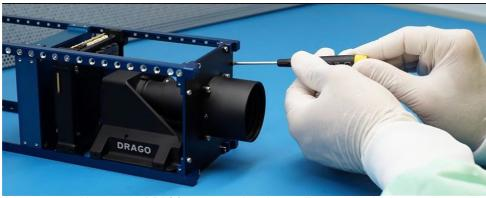
Mounting the DRAGO camera on the microsatellite structure simulator
