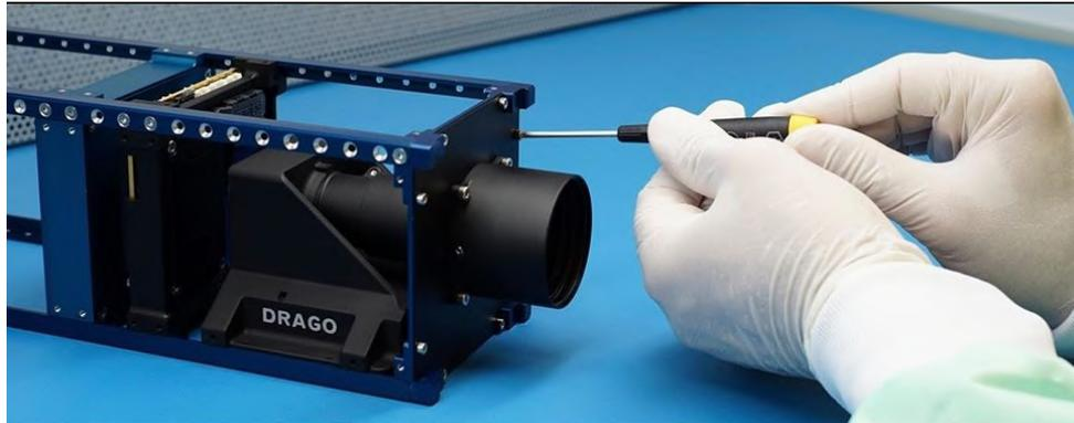
*Mounting the DRAGO camera on the microsatellite structure simulator*
