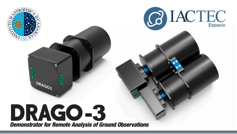
**DRAGO-3** is the third-generation instrument in the DRAGO family of space cameras developed by the IAC for Earth observation in the shortwave infrared (SWIR) spectrum. Building on the success of **DRAGO-1** and **DRAGO-2**, this new version includes a greater number of spectral bands and offers significant enhancements in resolution, sensitivity, and efficiency, along with a modular design tailored for integration into future satellite constellations.
